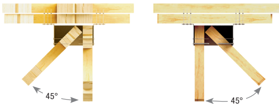
Typical HJC/HTHJ installation top view
