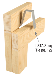
Additional strapping for high uplift
